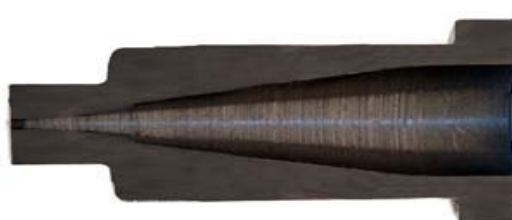
CROSS-SECTION OF A PVC NOZZLE
