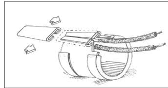
**Wedge Lock —** provides low profile clamping where space is limited and can not be used. Available in Type 3 or 4 leads.
