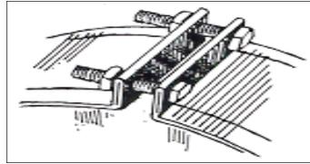
**Clamping Tabs –** Are available for applications where straps impede openings for instrumentation. However, high-torque clamping straps provide superior heat transfer and should be used whenever possible.
