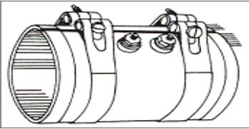
**Barrel Nut Strap – Standard Heater Construction.** High torque clamping straps provide superior heat transfer and greatest heater life; should be used whenever possible. Flexible strap locating allows for easier installation.
