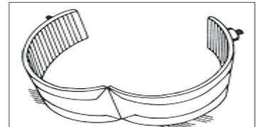
**Expandable Bands** are designed to be opened and closed for quick installation. They are shipped open and **should not be opened or closed more than twice.** Available in all lead options.
