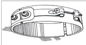
**Two Piece Bands** can be easily installed over a cylinder rather than slipped on from the end. Specify the line voltage and wattage per half. Available in all lead options.
